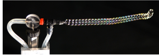
Figure 3 Example of mono-disperse bubble generation (here: fused bubble chain before flow-induced separation).
