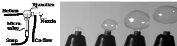
Figure 2 Left: Elements of the bubble generator. Right: Time lapse of bubble formation at the nozzle.
