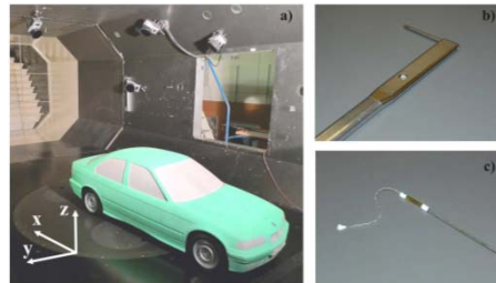
Fig 2: a) Motion capture system in the test section of the wind tunnel, b) Pitot-static probe. c) Tuft probe.
